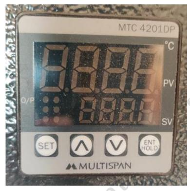
Figure 2: Digital temperature controller
